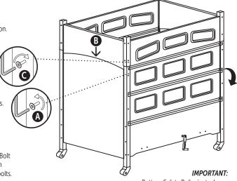
Bottom Safety Rail pivots down. Use both hands to carefully operate.
