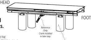
When placing cardboard lifts beneath foundation, allow room for both side panels to be attached.
