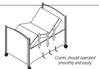
For Extensions, check operation of Safety Latch holding the top Safety Rail.
