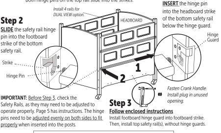
IMPORTANT: Once installed, use both hands to bring the safety rail up and attach it to the posts. Verify that it latches securely to both posts,
