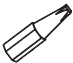
1) Torx Bit For use to adjust strike plate on safety rail if necessary.
