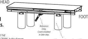
When placing cardboard lifts beneath foundation, allow room for both side panels to be attached.
