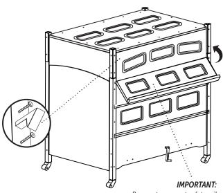
Be sure to support safety rail with both hands while moving the rail into their secure positions.
