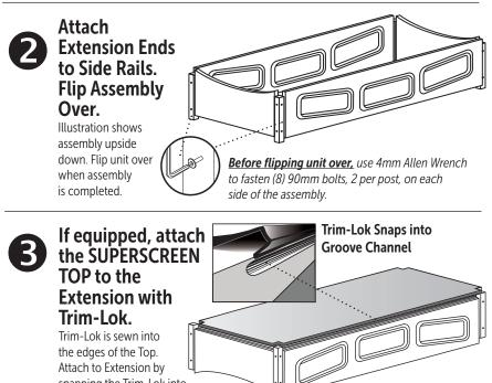
snapping the Trim-Lok into the grooves on the edge of the Extension.
