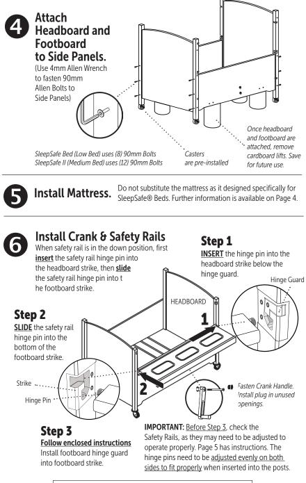
IMPORTANT: Once installed, use both hands to bring the safety rail up and attach it to the posts. Verify that it latches securely to both posts,
