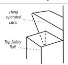
This latch should be properly mounted to the Extension to ensure top Safety Rail is securely held in place.
