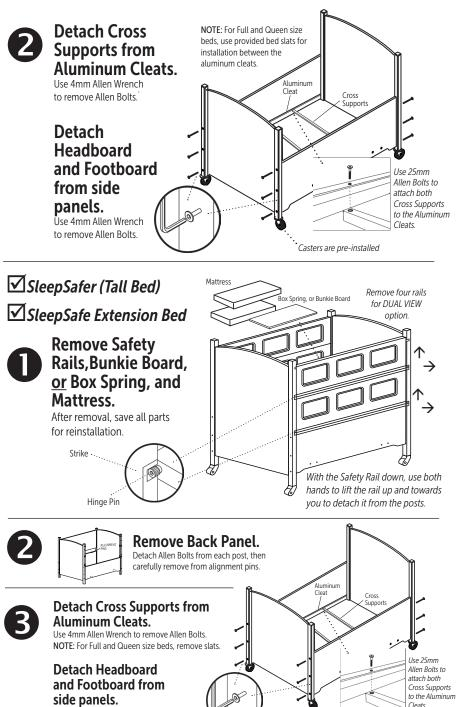
Use 4mm Allen Wrench to remove Allen Bolts.
