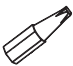
1) Square Bit For use to adjust strike plate on safety rail if necessary.
